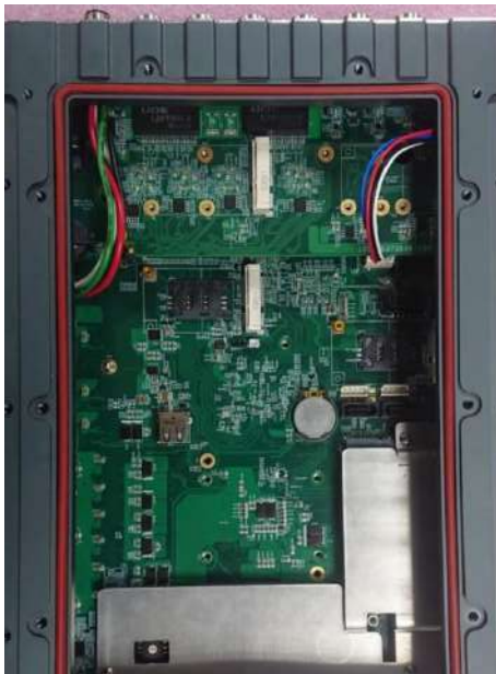
O-ring seated properly in the groove
