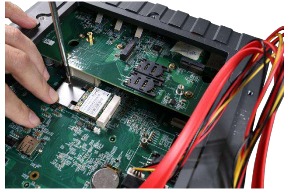
Secure the module with a screw
