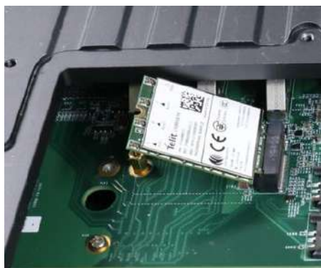
Insert into slot on a 45 degree angle
