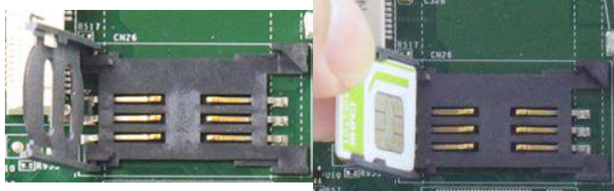
Slide and lift SIM card holder
