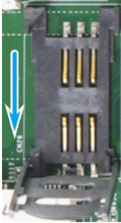
Slide and lift SIM card holder Insert SIM card with pins facing up
