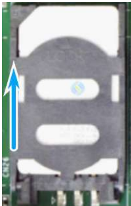
Slide and lift SIM card holder Insert SIM card with pins facing up
