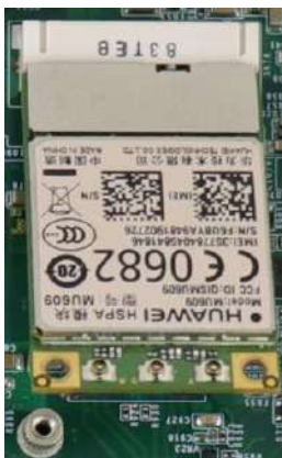
Insert at 45 degree angle Secure with a screw
