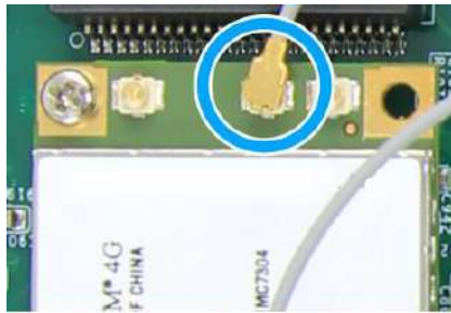
Clip on IPEX-to-SMA cable
